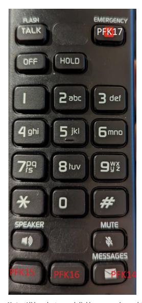
**Note**- All handset speed dial keys are mirrored to phone base speed dial keys. PFK 15 and 16 may be overridden to different destinations (See Configuration Module)
